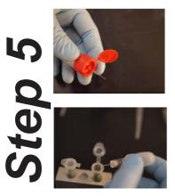
■ Take out a capillary tube which may be used the holder provided (pipette bulb); or it may be used by holding the capillary tube between your thumb and finger (be sure not to let the glove block the open end of the capillary tube in your hand or it will not draw the fluid up properly).
