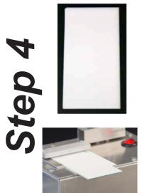
■ The test plate should be laid out with the coated side facing up, be careful not to touch the white front of the plate. The 5cm edges should be the bottom and the top edges, while the 10cm edges are the sides.
